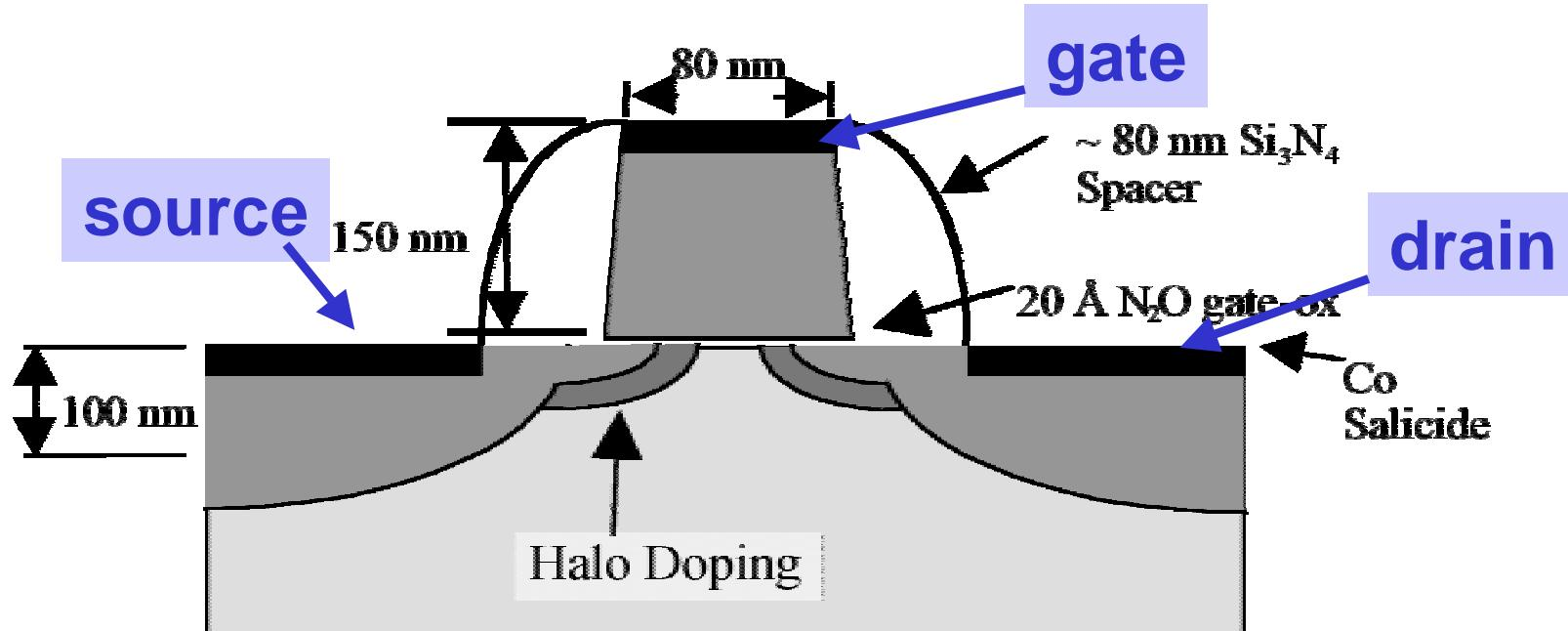
MOSFET – resistor + capacitor
