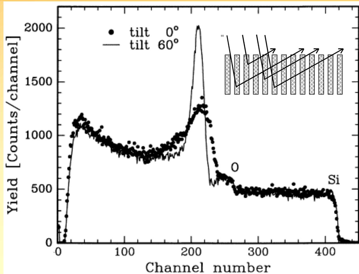
**R-BS spectra on columnar porous Si (3045+100 keV  ${}^4\text{He}^+$ ). The peak is due to  ${}^{16}\text{O}(\alpha,\alpha)$  resonance.
