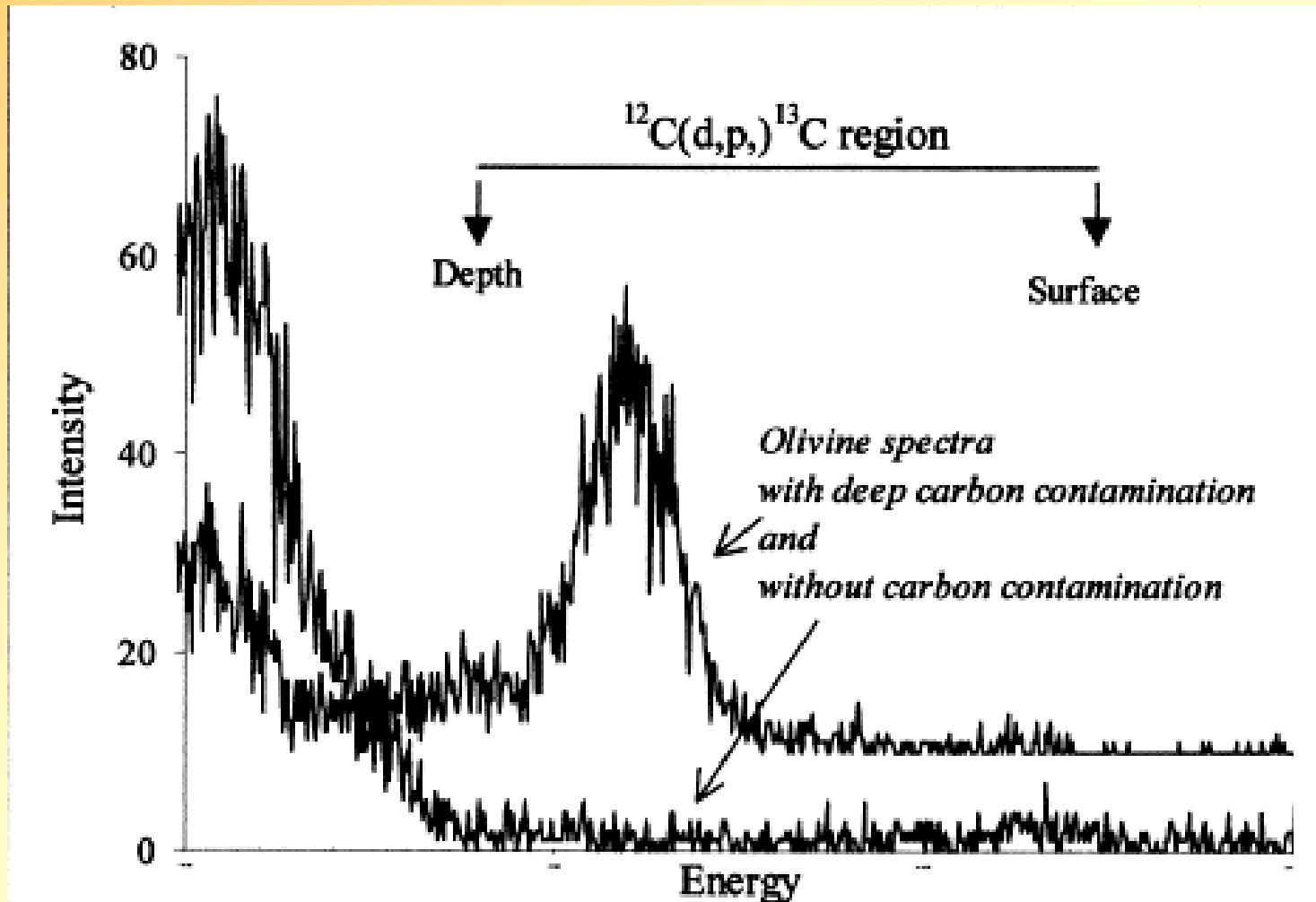
$^{12}\text{C}(\text{d},\text{p})^{13}\text{C}$  NRA spectra of olivine with 1000 ppm C content (1.45 MeV d, 9  $\mu\text{m}$  Al filter foil)
