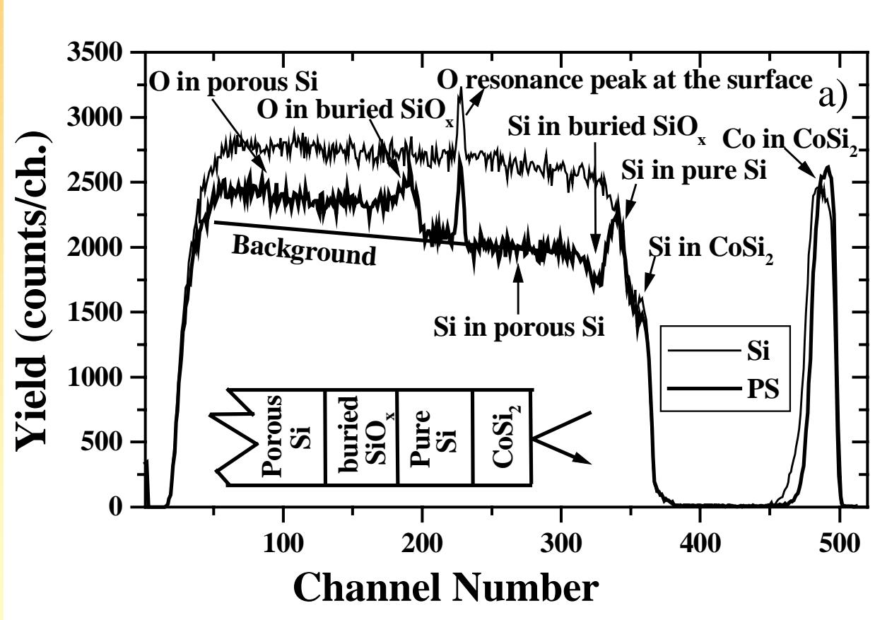
**RBS spectra (3.045 MeV  ${}^4\text{He}$ ) of Co implanted Si and a porous Si.**
