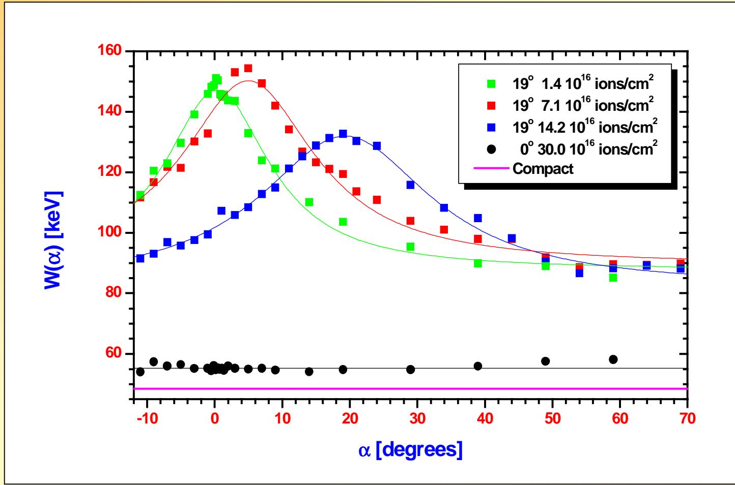
**Half-width of the resonance peak for samples implanted at various tilts and fluencies.**
