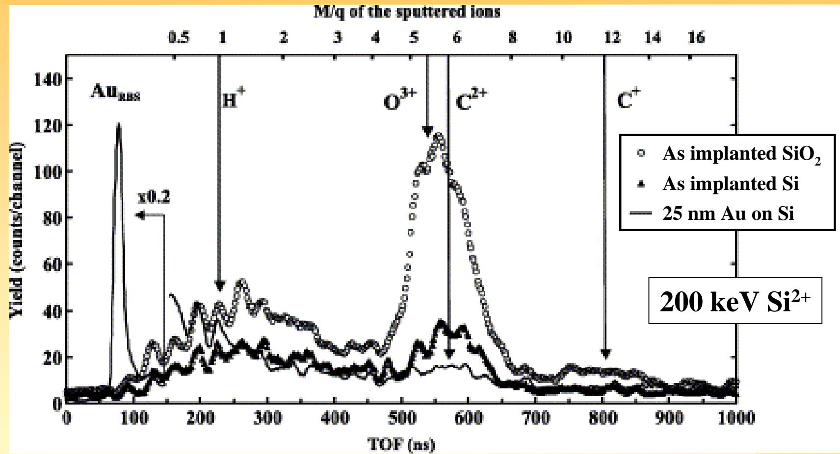
**TOF spectra by the 200keV FIB. H, O, C peaks are due to secondary ions accelerated by the 1.8 kV detector bias of the MCP (TOF-SIMS).**
