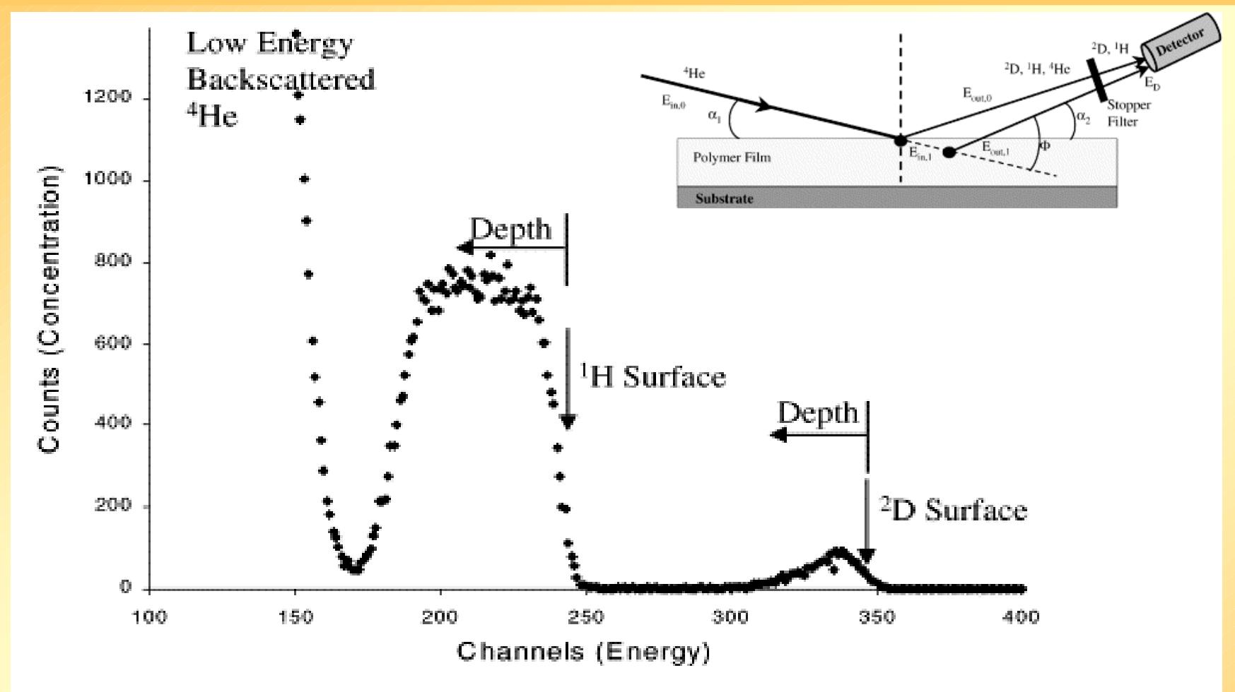
**ERD spectrum from a thin, 200 Å, deuterated polystyrene film**
