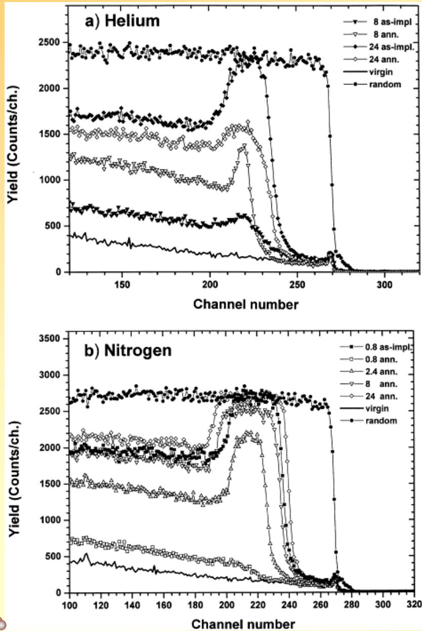
Channeling RBS spectra of He and N-implanted and annealed Si. Virgin and random spectra are also included.
