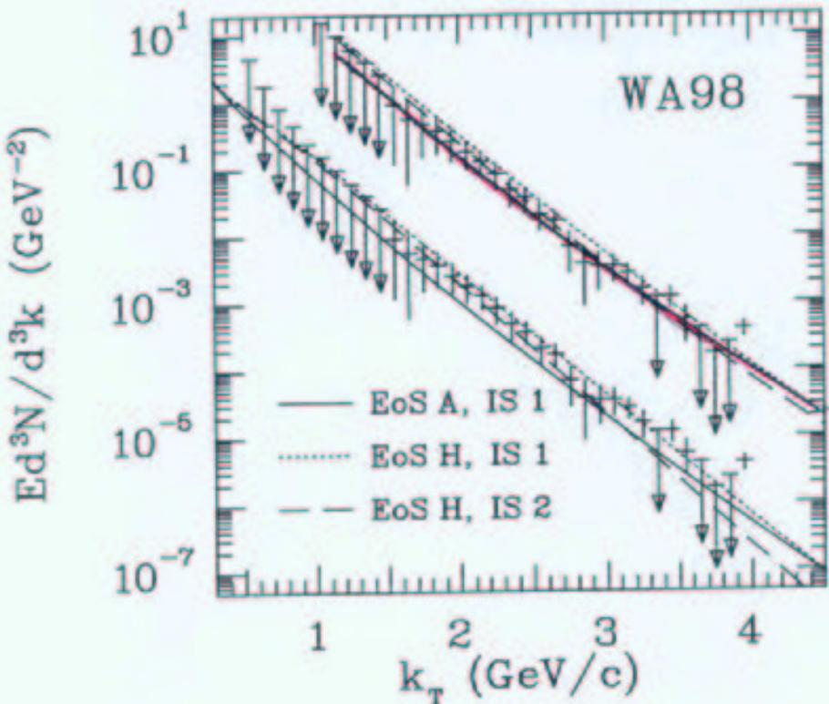
Thermal photon emission for different EoS and initial state with the contribution of initial pQCD photons (upper set, scaled by factor 100) and without (lower set).
