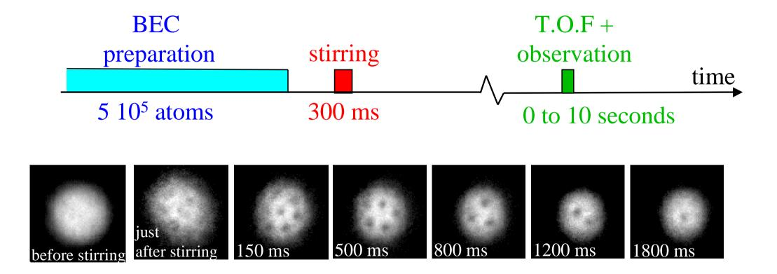
Different time scales for the decay of the array and of the last vortex (also at MIT) 2.
