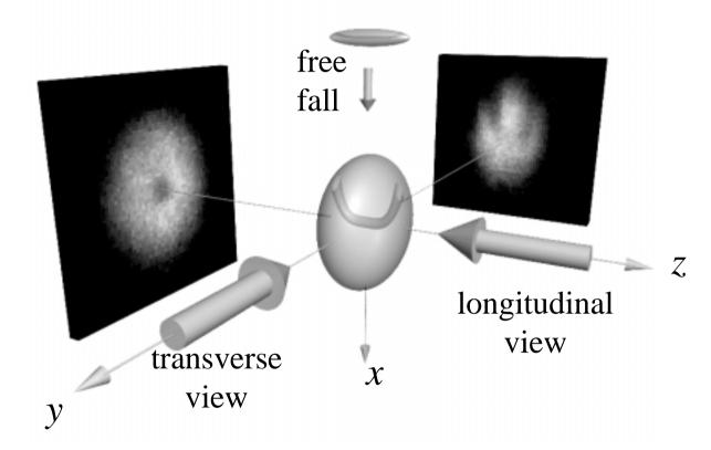
similar transverse imaging developed in Boulder and Oxford for a vortex array A single vortex line is generally not straight... U shaped or N shaped
